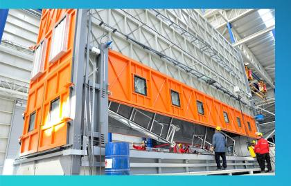
Keeping zinc fume generated during material dipping in a closed area
