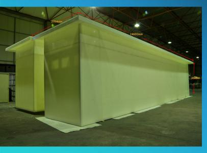
The possibility of manufacturing process tanks in one piece by using Wegener Machines installed in both factories,
